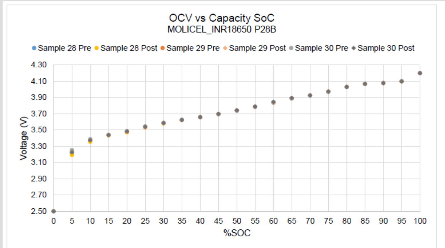
Figure 2.2.3.2 – Capacity vs Voltage at each 5% DoD.
