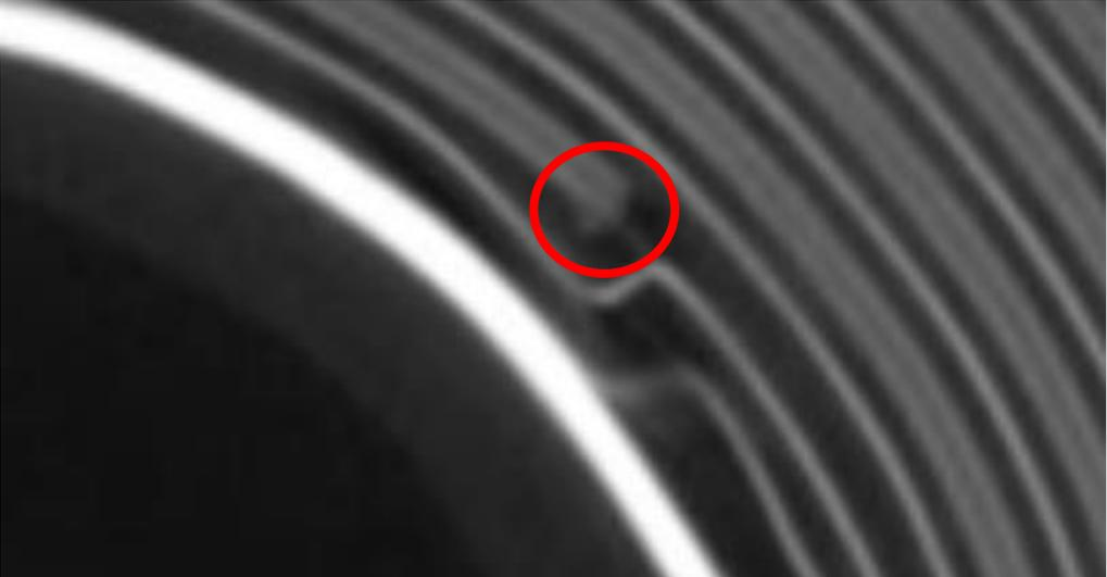
3 Fail - Delamination of Graphite (same image as #2 from slide #18)
