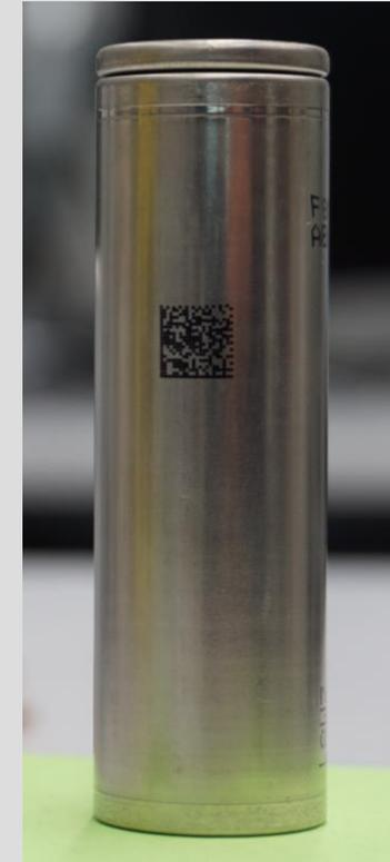
Samsung makes OCV data out to 4 decimal places available via QR code on each cell can
