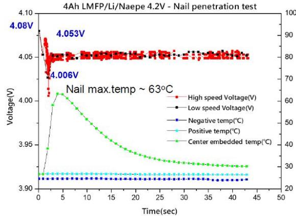
LMB Cell showed 74mV voltage drop at the beginning of nail penetration, then recovered to 27mV drop by the ISC fusing.
