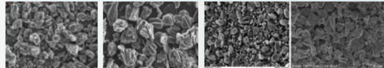
Conventional: 345 High capacity: 360 Si-based+graphite 550 SiO 1350,92%
