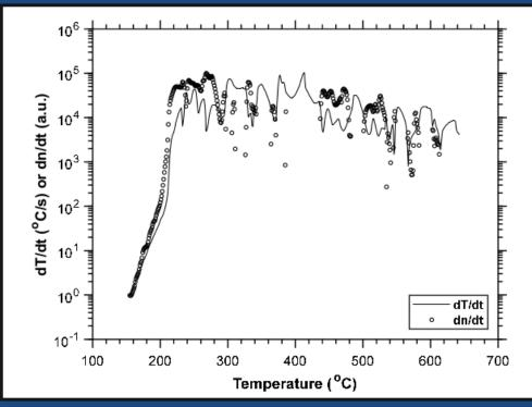
Cell heating rate and gas generation rate based on calorimetry measurements for an 18650 LCO cell (Ostanek et al., Jhu et al.)
