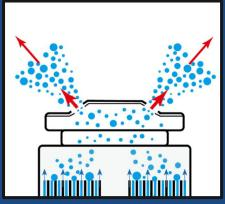
$V_h$  : Headspace Volume  $T_{cell}$ : Mean temperature of battery  $R_j$  : TR rxn rate of  $j^{th}$  rxn  $\Delta m_j$  : Mass of vent gas from  $j^{th}$  rxn
