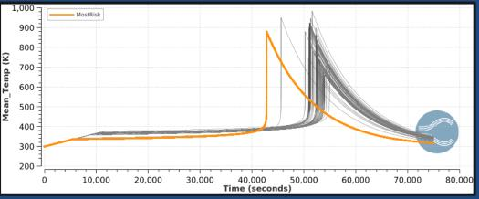
Worst case scenario : All cells modeled with MostRisk parameters Results in rapid TR propagation across entire battery pack
