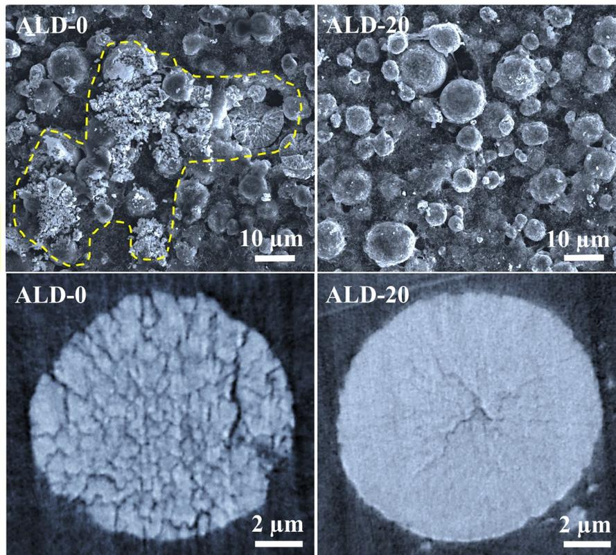
ALD  $\text{Li}_2\text{S}$  coating well protected NMC811 from cracking
