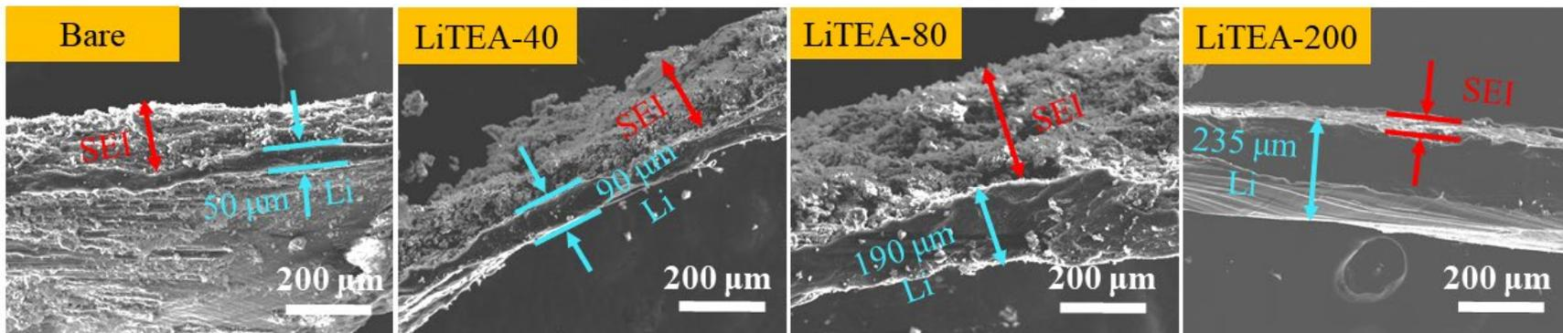
After 500 Li-stripping/plating cycles at 2 mA/cm<sup>2</sup> and 1 mAh/cm<sup>2</sup>.
