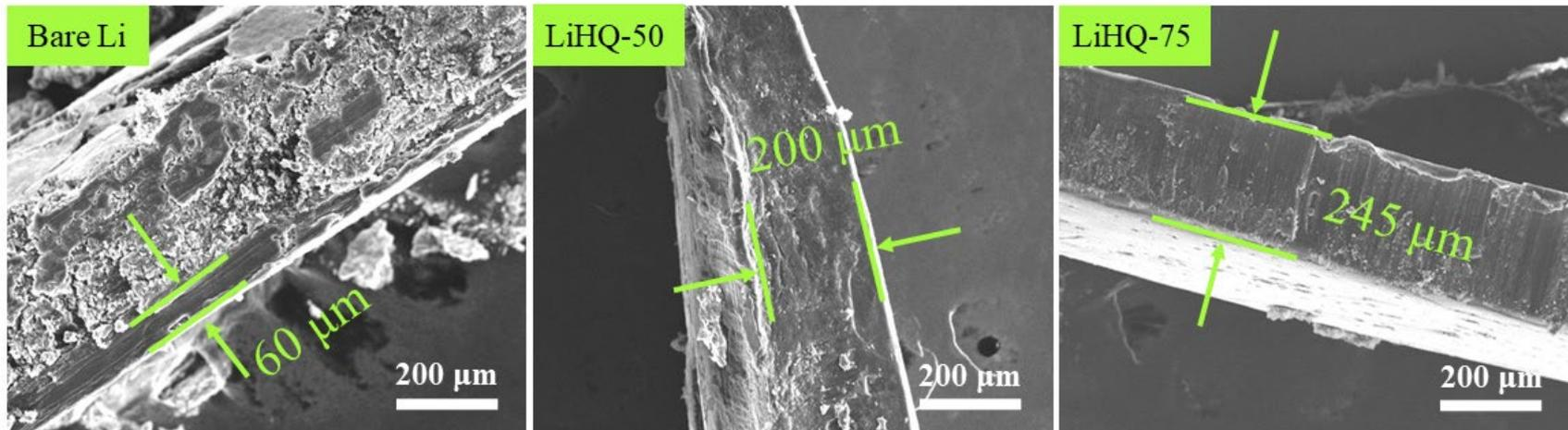
After 500 Li-stripping/plating cycles at 2 mA/cm<sup>2</sup> and 1 mAh/cm<sup>2</sup>.
