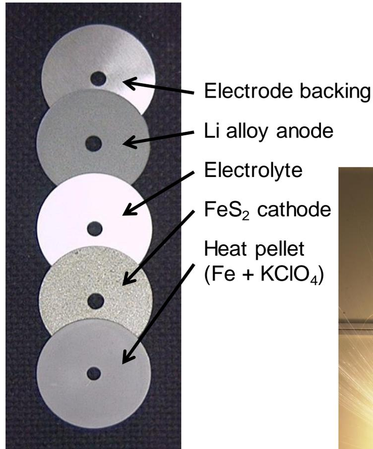
Current pulse through pyrotechnic initiator (squib) ignites heat pellets through centerline, activating battery
