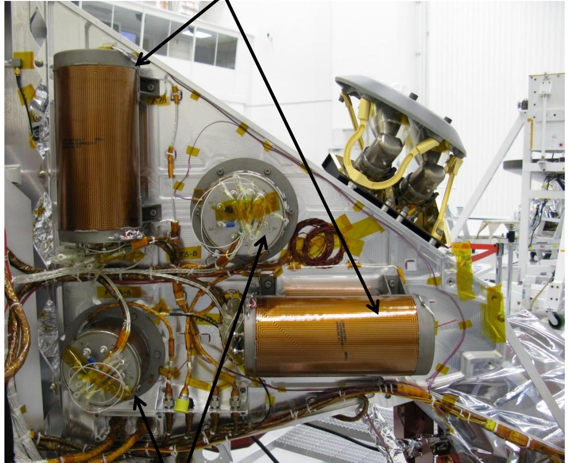
Pyro Thermal Batteries (PYTBs)
