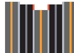
Insufficient electrode overhang
