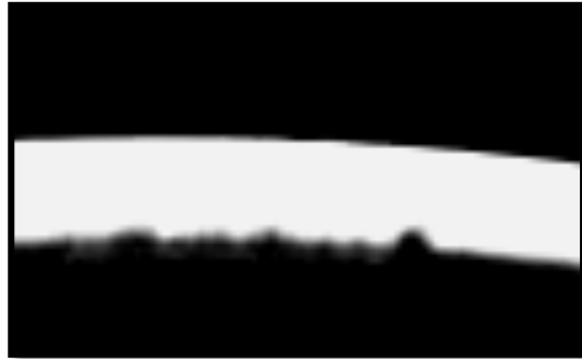
Pits in cell cap crimp area
