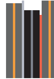
Missing/insufficient separator overhang
