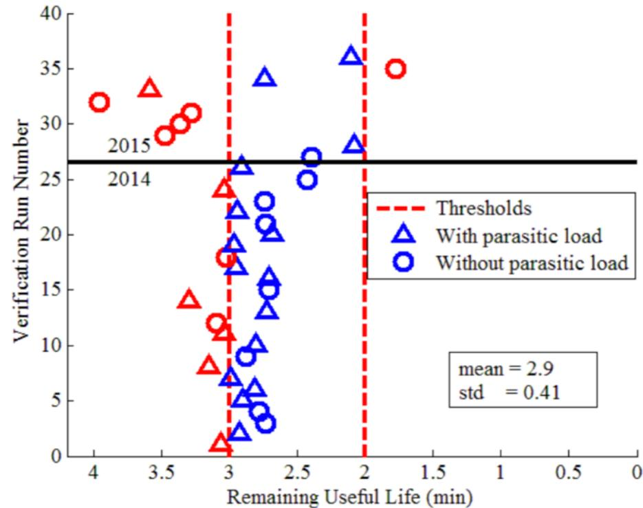
Two-minute alarms for additional runs done a year later using updated battery capacity parameters.
