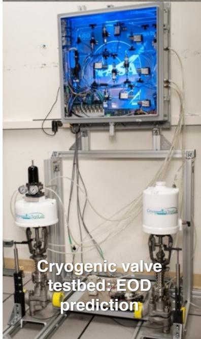
Cryogenic valve testbed: EOD prediction
