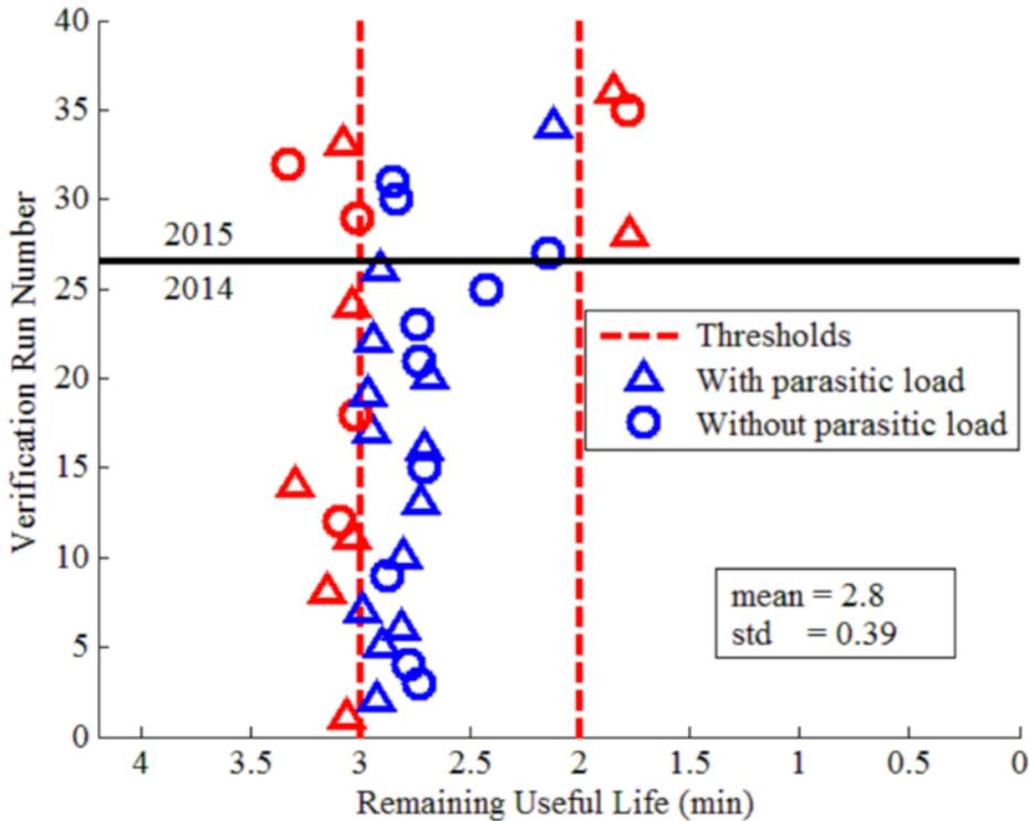
Two-minute alarms for additional runs done a year later using out-of-date battery capacity parameters.
