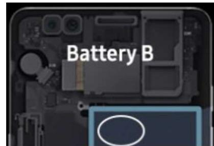
Check insulation tape status 100% vision check is mandatory during the manufacturing process. QC checks it every batch and many inspections.
