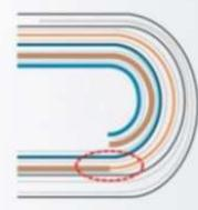
The tip of the negative electrode is correctly located within the planar arena
