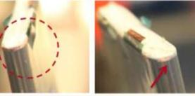
REPEATED DEFORMATION PATTERNS CAN BE OBSERVED AT THE CORNERS OF THE SEPARATOR
