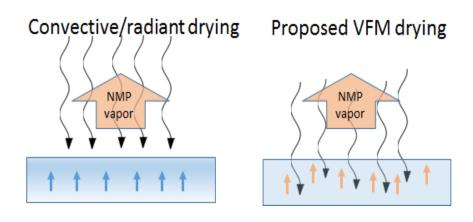
Compared to baseline convective electrode drying, VFM transfers energy to the electrode bulk, vaporizing NMP (orange) and avoiding dragging electrode binder (blue arrows) which creates a gradient with low binder content at the current collector interface.
