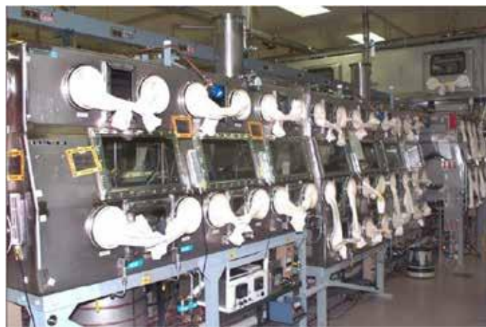
FIGURE 3-23 | AQUEOUS PROCESSING GLOVEBOX LINE AT LANL
