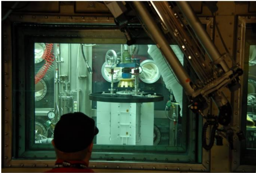
FIGURE 3-25 | MMRTG BEING ASSEMBLED IN IAAC
