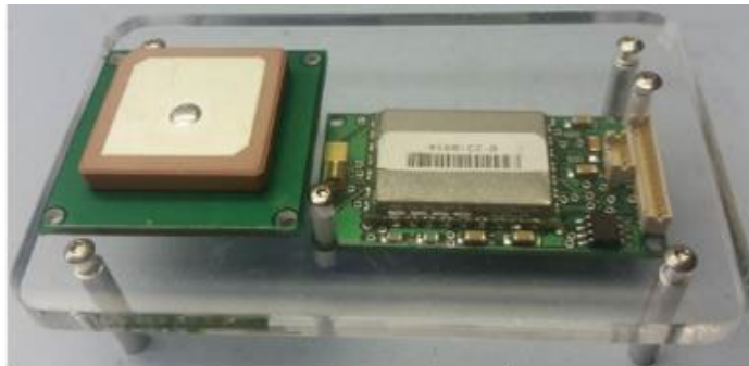
Simplex: STX-3 (or STX-2): 200 Kbytes/day, 9 Bytes/sec
