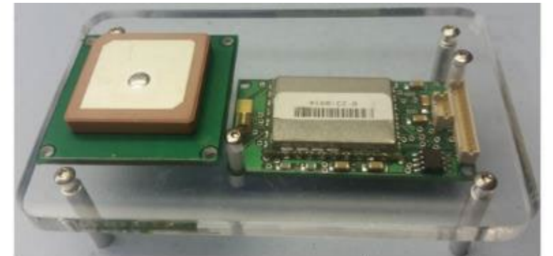
Simplex: STX-3 (or STX-2): 200 Kbytes/day, 9 Bytes/sec
