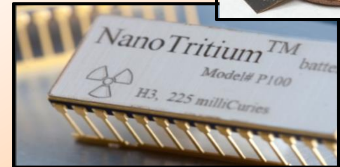
NanoTritium™ - City Labs USNRC Registered: General License for Model P100-P200 (up to 100 Curies)
