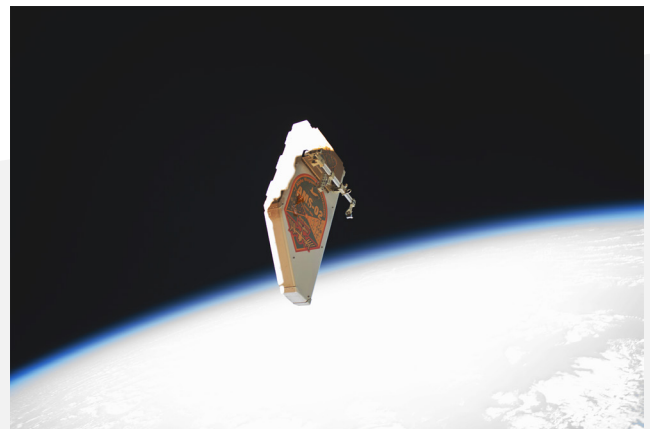
Front image: A debris shield that was removed from the Alpha Magnetic Spectrometer (AMS), the International Space Station's cosmic particle detector, is pictured drifting away from the orbiting lab after spacewalkers Andrew Morgan and Luca Parmitano jettisoned it. The debris shield was detached by the spacewalkers so they could access and begin the repairs of the AMS thermal control system.
