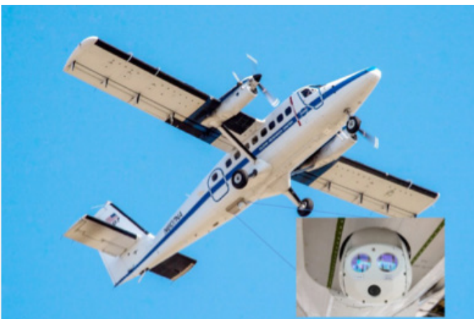
Figure 19: 1GRC Airborne Laser Communication Testbed in flight aboard the GRC DHC-6 Twin Otter Aircraft.
