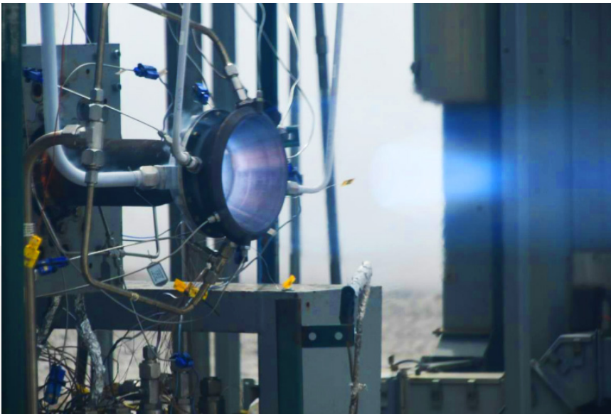
Figure 1: Successful hot-fire test of a liquid oxygen/methane (LOX/LCH4) injector and nozzle using new NASA alloy GRX-810. The GRX-810 alloy has incredible performance benefits in extreme environments and was featured in 2023 in Nature Magazine. NASA's center chief technologists champion such efforts in the agency and assist execution of funding programs to develop breakthrough advances.
