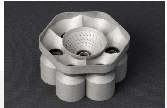
Figure 2: This turbine engine combustor (fuel-air mixer) was 3D-printed at NASA Glenn Research Center (GRC) and is one example of a challenging component that can benefit from applying a new alloy called GRX-810. The NASA alloy GRX-810, an oxide dispersion strengthened (ODS) alloy, can endure temperatures over 2,000 degrees Fahrenheit, is more malleable, and can survive more than 1,000 times longer than existing state-of-the-art alloys. This new alloy can be used to build aerospace parts for high temperature applications, like those inside aircraft and rocket engines, because ODS alloys can withstand harsher conditions before reaching their breaking point.
