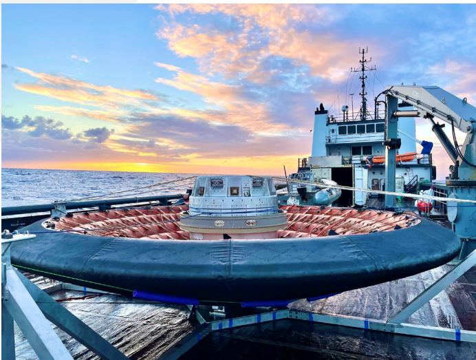
Figure 24: The Low-Earth Orbit Flight Test of an Inflatable Decelerator, or LOFTID, spacecraft is pictured after its atmospheric re-entry test in November 2022.
