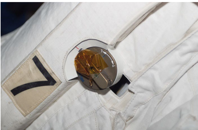
STS-121 SAFER latch taped with Kapton tape
