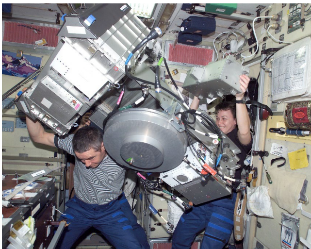
Cosmonaut Valery Korzun and astronaut Peggy Whitson perform maintenance on the Treadmill Vibration Isolation System (TVIS) in the Zvezda Service Module on the ISS. Photo: NASA (2002)
