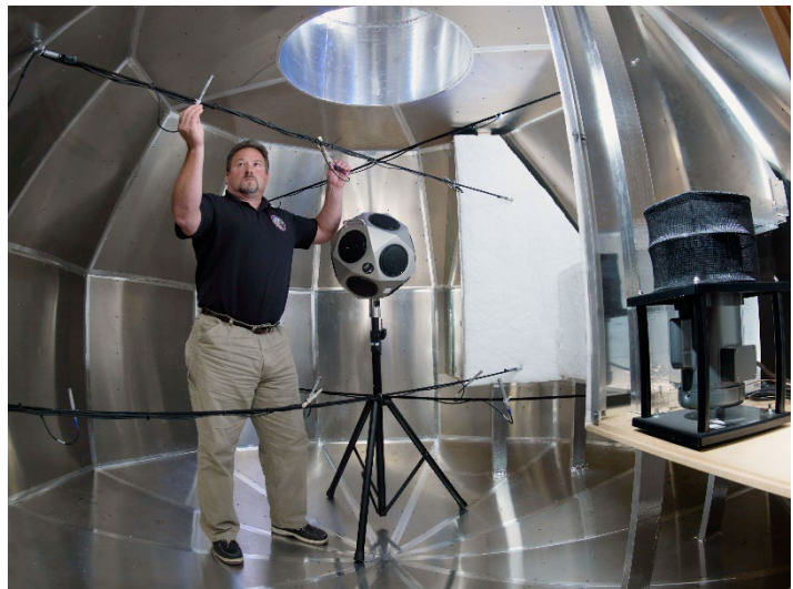
An acoustic engineer validates the Multi-Purpose Crew Vehicle Command Module Volumetric Acoustic Mock-up.
