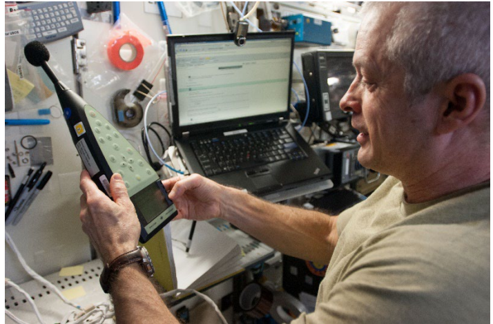
ISS crewmember performs Sound Level Meter (SLM) Operations to measure the acoustic environment in the ISS.
