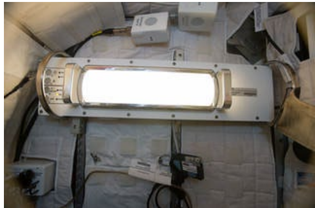
Solid-State Lighting Assembly
