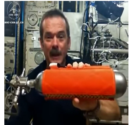
U.S. Portable Fire Extinguisher on ISS
