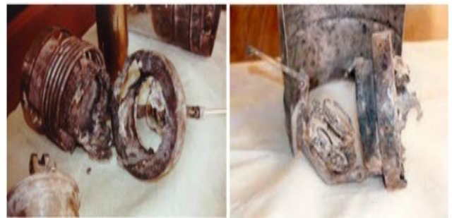
Charred remains of the solid fuel oxygen generator returned from space station Mir
