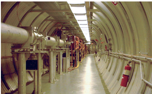
The Phantom Torso is used on the ISS to detect and measure neutron radiation (above). A radiation beam line is used to gather data on effects from exposure to high-energy particles (left).
