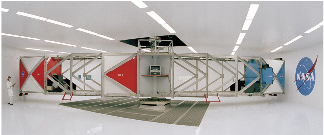
The 20-G Centrifuge, used for hypergravity research at the Center for Gravitational Biology Research.
