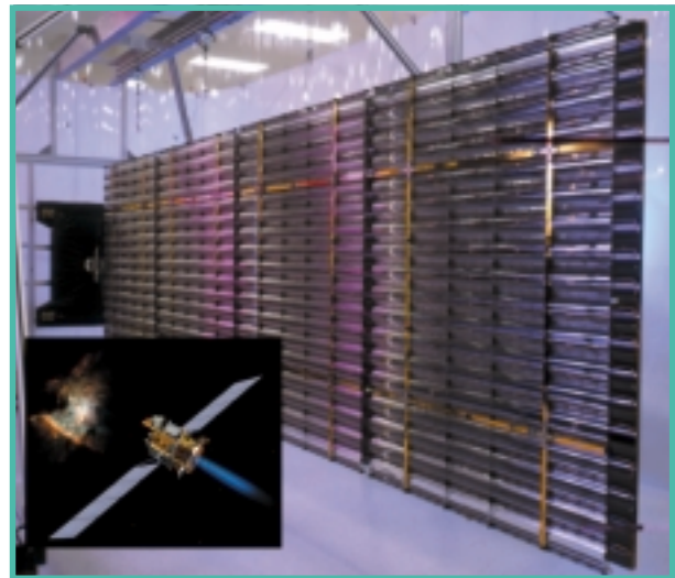
GRC solar concentrator array with refractive linear element technology (SCARLET) used on Deep Space-1 spacecraft (inset).
