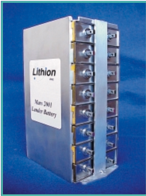
Prototype lithium ion battery selected for NASA's Mars 2001 mission.
