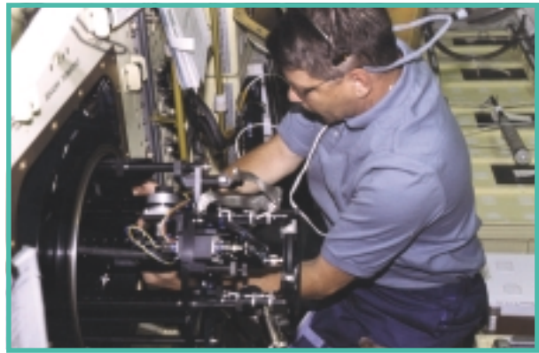
Installation of GRC Laminar Soot Processes Experiment on Space Shuttle Mission MSL-1.
