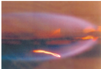
The Forced Flow Flame-Spreading Test was designed to study flame spreading over solid fuels when air is flowing at a low speed in the same direction as the flame spread.
