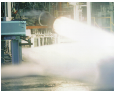
Test of the low-cost Fastrac rocket engine.
