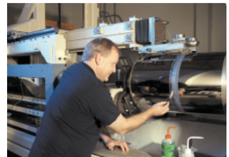
Precision polishing of 0.5 m Constellation X-ray mandrel.
