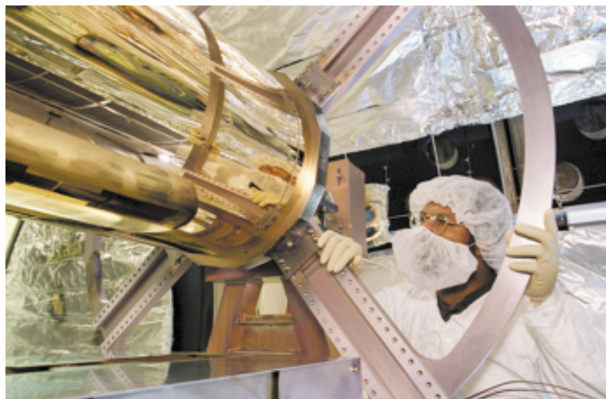
Precision coating of 05-m Constellation X-ray mandrel in Large Coating Chamber.
