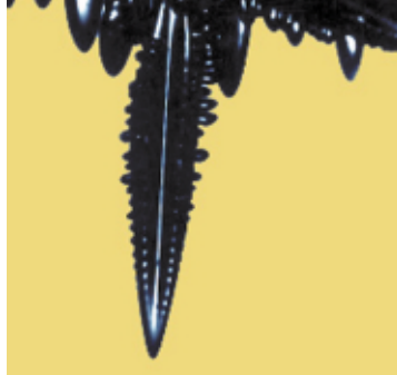
Dendrites, which are materials microstructures, are frequent objects of study in microgravity.
