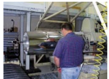
50-cm x-ray mandrel for diamond turning.
