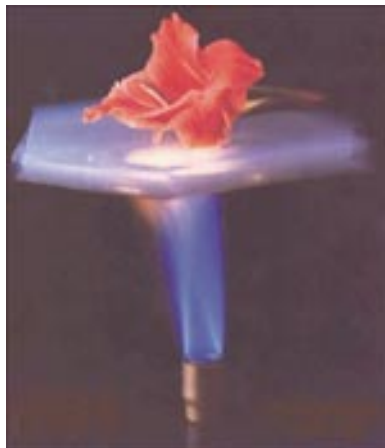
Aerogel insulation protection properties are capable of shielding a delicate flower from intense heat.
