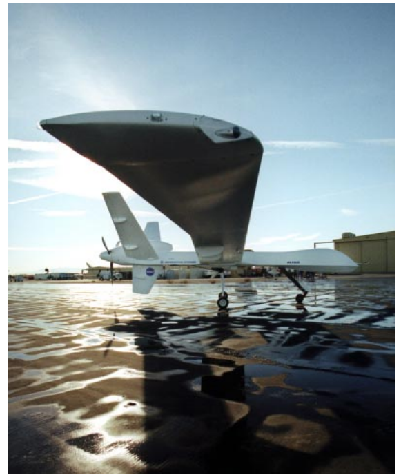
The Altair Unmanned Aerial Vehicle shows off its lengthy high-aspect ratio wing. Photo by: GA-ASI/Alan Waide
