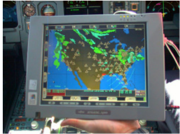
NASA graphical cockpit weather displays provide real time information that can help aircrews avoid areas of hazardous weather.
