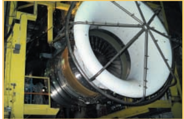
PW4000 low-nitrogen-oxide engine combustor test.
