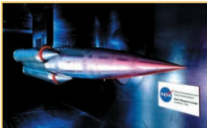
GTX model tested in GRC 10-by 10-Foot Supersonic Wind Tunnel.
