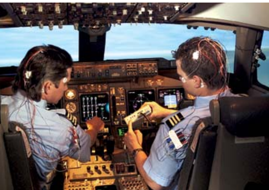
(above) Pilot brain wave activity is monitored in the Crew Vehicle System Research Facility's Boeing 747-400 Simulator during a study to determine fatigue, sleep loss, and circadian rhythm disruption during long- and extra-long-haul flights. Fatigue is measured during flight simulations to discover better ways to counter the adverse effects of fatigue on flight crews.
