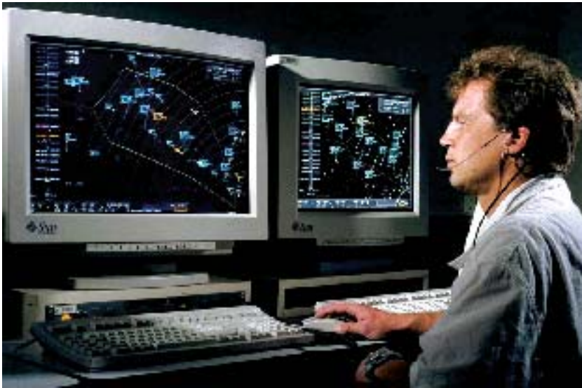
(above) Controller using Center/TRACON Automation System (CTAS) tools to plan an efficient arrival flow into a busy terminal area.
