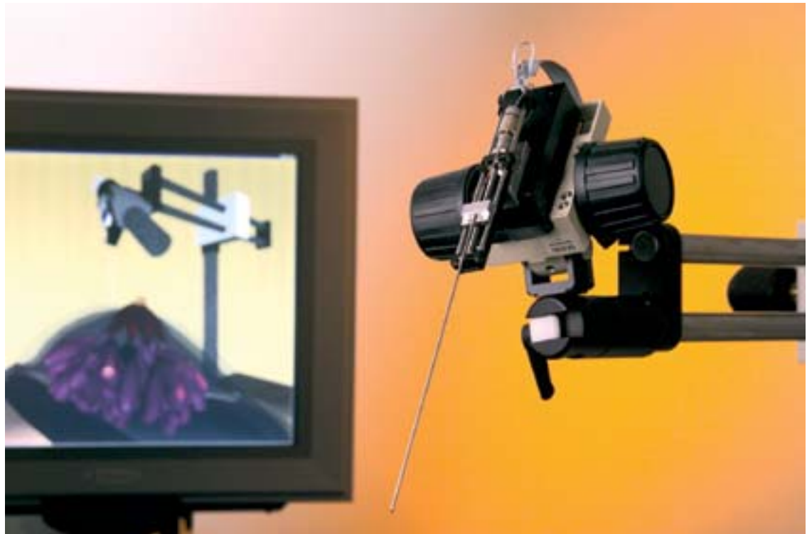
(right) The Smart Surgical Probe is a small disposable needle with multiple sensors that can simultaneously measure multiple physiological parameters within a breast tumor. This process is a major advancement in the state of the art of breast cancer detection. The probe, developed at Ames in partnership with Stanford University School of Medicine, was patented and licensed.
