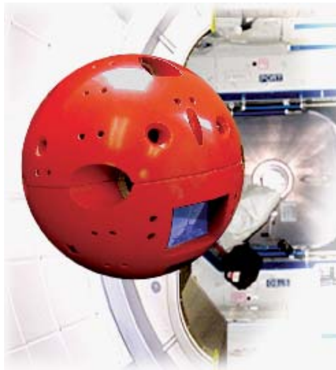
(above) The Personal Satellite Assistant is a small astronaut support device designed to assist astronauts who are living and working aboard the Space Shuttle, Space Station, and during future space exploration missions.
