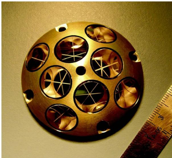
LRA has eight retroreflectors inside. It will be mounted on Astrobotic's Peregrine lander deck and help provide precision measurements of distances between orbiting or landing spacecraft. *Credit: NASA*
