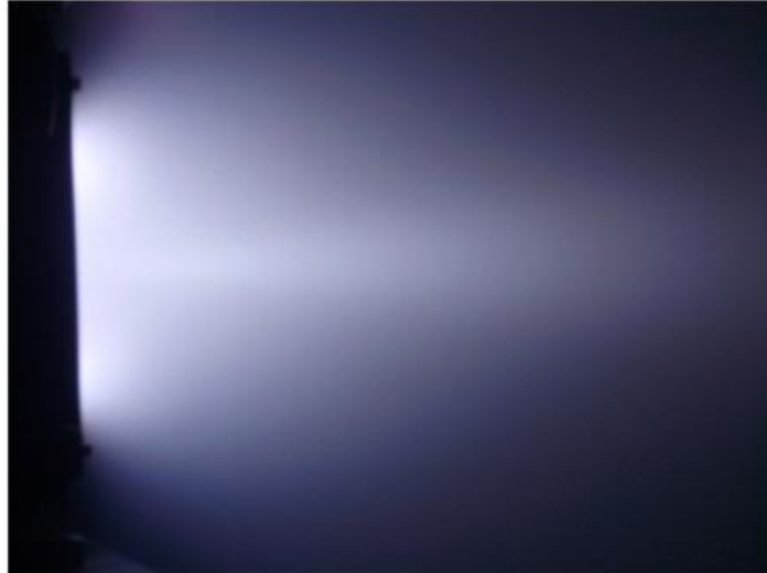
Figure 3 Hall thruster running on CO 2 in Busek facility
