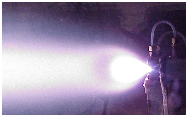
Figure 22 Busek arcjet operating in free jet mode
