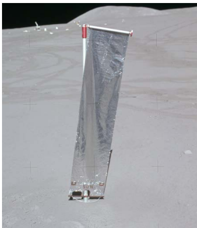
Figure B9 – Solar Wind Composition Experiment (Only Support Pole Remained on Moon)
