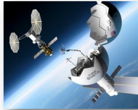
ThinkOrbital – A system to robotically assemble and weld very large pressurizable modules for CLDs in-space
