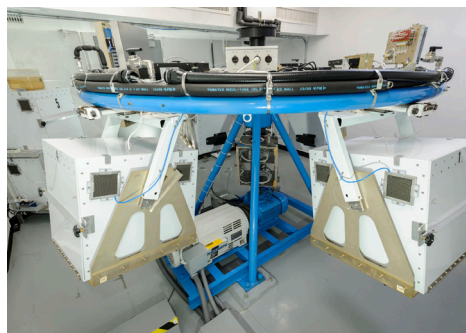
1.22-Meter Radius Centrifuge
