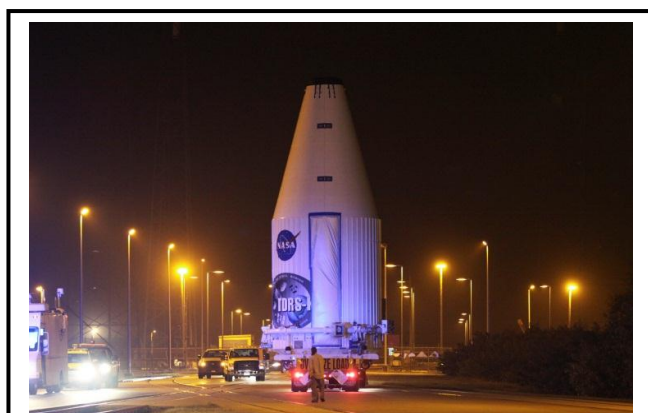
Enclosed in its payload fairing, NASA's Tracking and Data Relay Satellite K, passes through the Launch Complex 39 area at Kennedy Space Center to its launch site. The spacecraft is part of the next-generation series in NASA's constellation of space-based communication satellites that provide tracking, telemetry, command, and high-bandwidth data return services.
