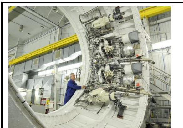
A technician performs a final check on the solid rocket booster avionics test article for in preparation for the second flight control test of NASA's Space Launch System at the ATK facility in Promontory, Utah. These avionics and boosters will be part of the first two flights of the Space Launch System – America's next heavy-lift launch vehicle managed by NASA's Marshall Space Flight Center in Huntsville, Alabama.
