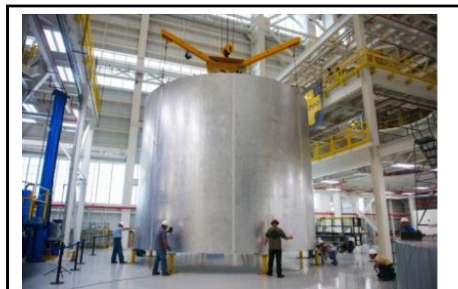
NASA finished welding the first “pathfinder” barrel section for the SLS core stage at Louisiana’s Michoud Assembly Facility in July 2013. The core stage will consist of eight stacked barrel sections for a total height of 211 feet. While the launch system will be over three times more massive than the Space Shuttle external tank, advanced manufacturing techniques will reduce the number of major tools and labor by more than 50 percent.
