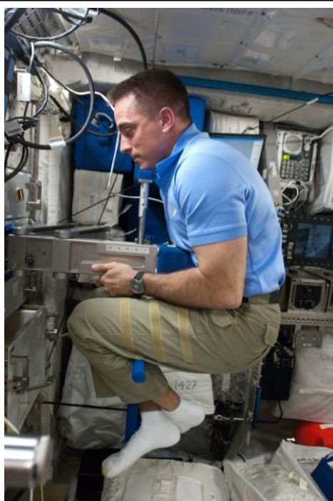
On April 8, 2013 on the International Space Station, astronaut Chris Cassidy, Expedition 35 flight engineer, weighs in using the Space Linear Acceleration Mass Measurement Device in the Columbus European Laboratory. Since crewmembers cannot weigh themselves in zero gravity, they use this method as the next best thing. Skylab astronauts, the first crewmembers to fly in space for over a month at a time some 40 years ago, used a body mass measurement device that was somewhat different from this. Prolonged spaceflight has a variety of effects on the human body and monitoring weight and especially weight loss is an important measurement that needs to be accomplished and documented.
