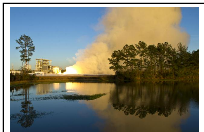
Engineers conduct a test of the Orbital Sciences Corporation Aerojet-Rocketdyne AJ-26 engine at Stennis Space Center in Mississippi. The AJ-26 is a modified version of the Russian NK-33 engine, which has been out of production since the end of the Soviet manned lunar program. Orbital refurbished the NK33 engines, and in September, the AJ-26 powered their Antares rocket from Wallops Flight Facility in Virginia. The launch marked Orbital’s final demonstration flight, and the maiden voyage of its Cygnus cargo vehicle. Developed as a part of NASA’s Commercial Orbital Transportation Services program, Cygnus delivered student experiments, food and supplies to the International Space Station, paving the way for future commercial resupply missions.
