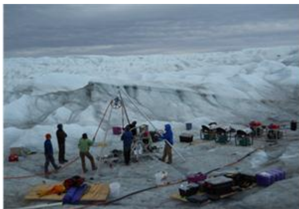
Researchers and students from University of Montana prepare to hot-water drill to the bottom of the Greenland ice sheet. They use measurements made in the boreholes to constrain numerical simulations of the ice motion. Airborne radar measurements provide critical additional constraints of ice sheet geometry and internal layering from the NASA IceBridge mission.
