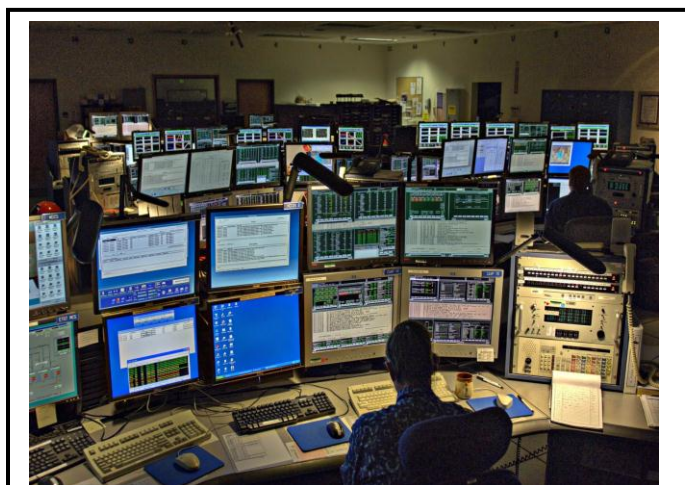
Operators manage Space Network ground and space assets at the White Sands, New Mexico complex, where data from orbiting satellites and the International Space Station are received and forwarded. Commands and other services such as voice and video are also transmitted from the complex to orbiting spacecraft. The Space Network operates 24 hours a day, 7 days a week to ensure continuous communication with the Station.
