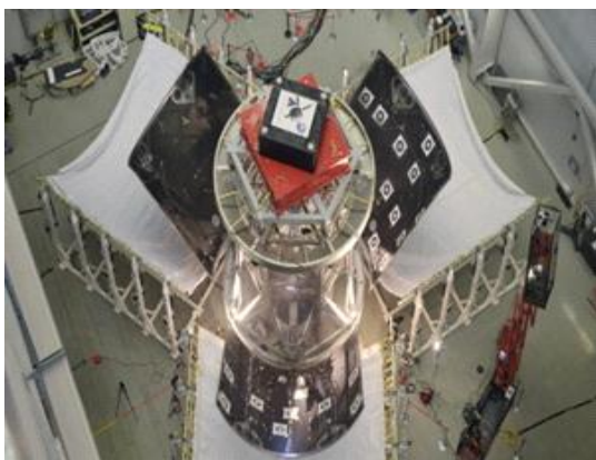
Three panels protecting NASA's Orion from the heat, wind, and acoustic loads it will experience during the early part of the climb into space fall away during a successful separation test. The panels jettison as Orion climbs out of the atmosphere to reduce weight and allow Orion to reach orbit.
