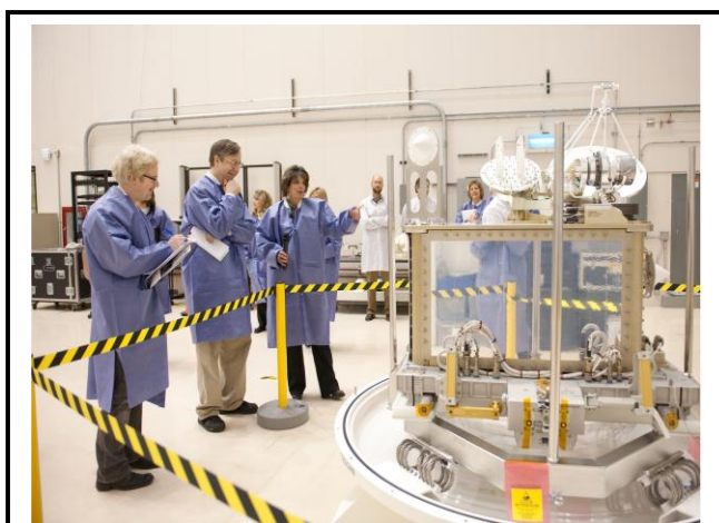
The SCA testbed, installed on the International Space Station last year, is seen here in the integration and test facility at the Glenn Research Center in Ohio. The testbed is demonstrating new radio technologies and navigation techniques using software-defined radios. Through a joint effort with the Department of Defense to monitor new Global Positioning System navigation messages, the testbed has already led to improvements in the system.
