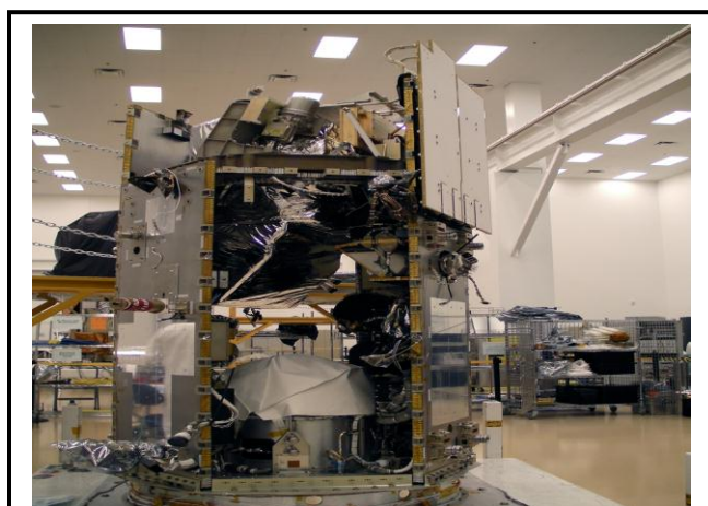
The Orbiting Carbon Observatory-2 (OCO-2) is comprised of a single instrument that flies on a dedicated spacecraft. The instrument, consisting of three high resolution grating spectrometers, will acquire precise measurements of atmospheric carbon dioxide. This image shows OCO-2 Observatory going into thermal vacuum testing.
