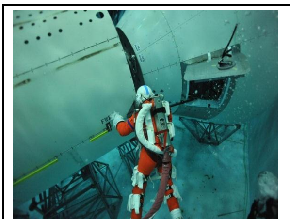
AES performs extravehicular activity (EVA) suit testing in NASA's Neutral Buoyancy Laboratory at JSC with the modified advanced crew escape suit – a concept for capsule-based EVA. Advanced space suit development enables humans to conduct "hands-on" surface exploration and in-space operations outside habitats and vehicles, and advances technologies such as portable life support systems, thermal control, power systems, communications, avionics, information systems, and space suit garments.
