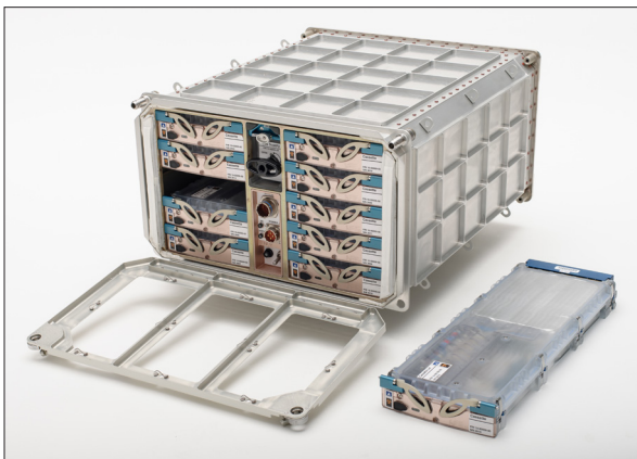
Bioculture System shown with one of the Cassettes removed. (Image credit: NASA / Dominic Hart)
