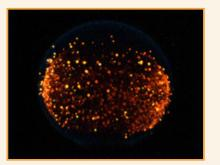
and produces larger bubbles, allowing scientists to observe and measure effects that are too fast and too small on Earth and providing a more complete understanding of heat transfer during boiling. This information could be applied to **cooling** electronics such as laptops more efficiently.
