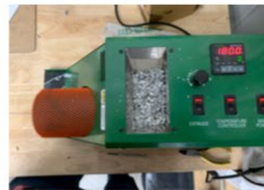
Shredded and Milled Catalyst-Infused ABS pieces in Filabot Hopper before Filament Extrusion
