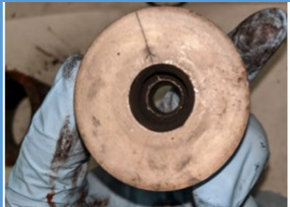
Thermally Induced Stress Failure of HBN Layer, Gen-1 Nozzle after 15-sec Burn
