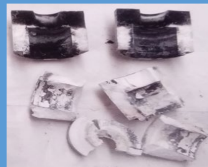
Thermally Induced Stress Failures of HBN Layer, Gen-2 Nozzle after 15-sec Burn
