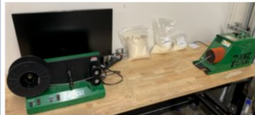
Filabot with Extruded Feedstock Filament
