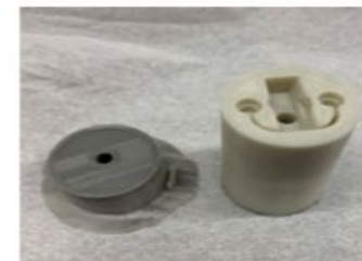
Plain ABS Fuel Grain, Ignition Slots, and Catalyst Insert with 2% Ru/Al 2 O 3 Infusion
