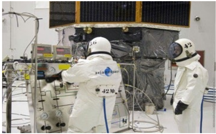
ESA technicians load hydrazine on the Herschel Space Observatory
