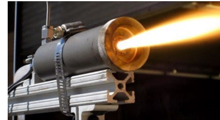
Sample ABS, FDP-Printed Fuel Grain
