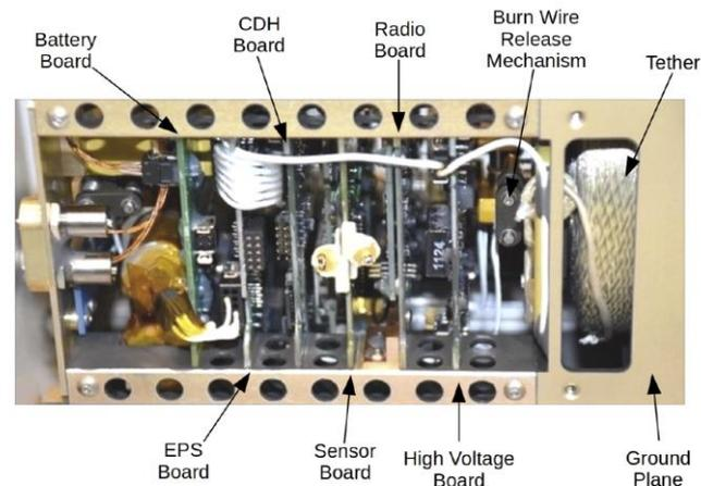
TEPCE Board Stack, Tether, Collector Tape, and Filaments
