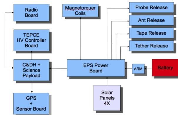
End-Mass Electronics Block Diagram
