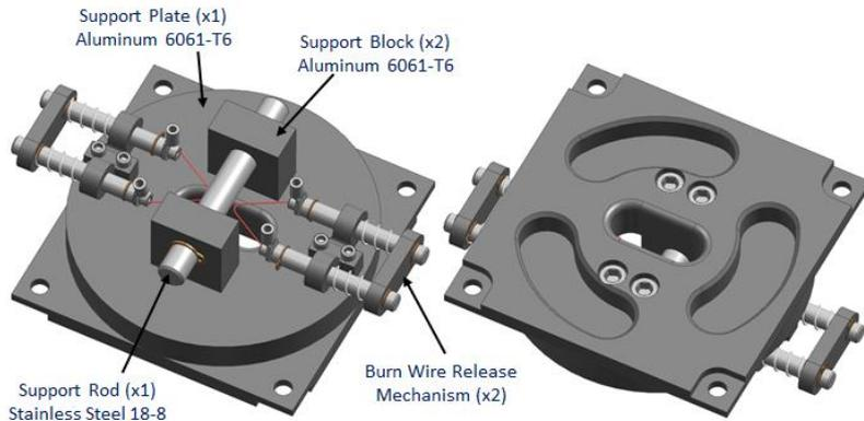
Stacer Release Mechanism
