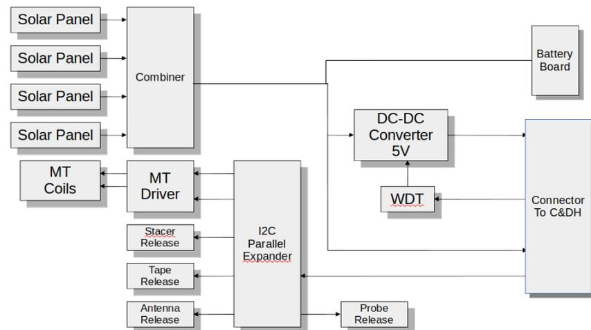
Electrical Power System Block Diagram
