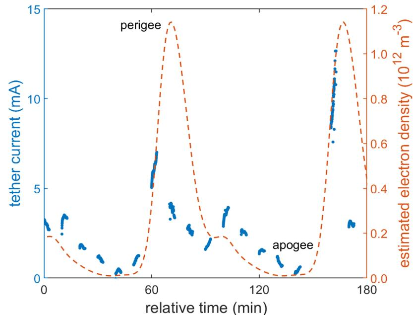
Measured Tether Current and Estimated Plasma Electron Density Over Approximately Two Orbits, Taken Dec 6, 2019
