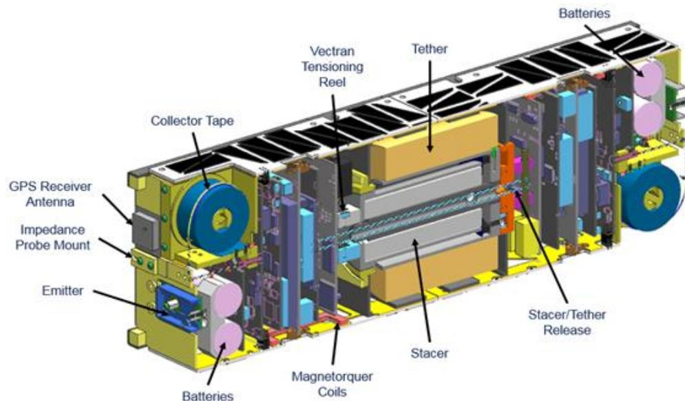
CAD Cutaway Drawing of TEPCE
