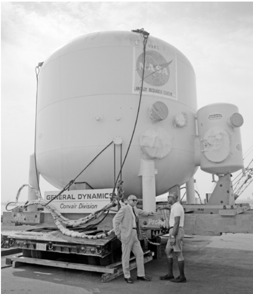
The $2.3 million ILSS arrives at Langley by barge from its manufacturer, the Convair Division of General Dynamics, in August 1965. Below is the home of the huge, 30-ton life-support tank in Building 1250. Test subjects occupied this facility for as long as 28 days at a time.
