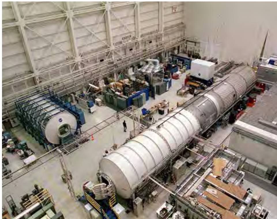
Marshall Space Flight Center designed and built the life-support systems that provide the crew of the International Space Station with clean air and water and a comfortable, safe work environment. The simulators shown here were used to develop the closed-loop system that allows the crew to recycle water and air aboard the station.
