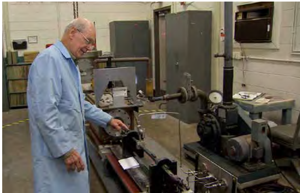
Don Humes, a retired NASA researcher who spent his 44-year career at NASA's Langley Research Center, points to the diaphragm separating the first and second stages of the Langley Miniature Light-Gas Gun. The breech of the 220 Swift rifle that serves as the first stage is clearly visible in the foreground.
