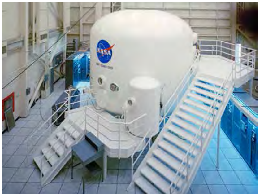
The $2.3 million ILSS arrives at Langley by barge from its manufacturer, the Convair Division of General Dynamics, in August 1965. Below is the home of the huge, 30-ton life-support tank in Building 1250. Test subjects occupied this facility for as long as 28 days at a time.
