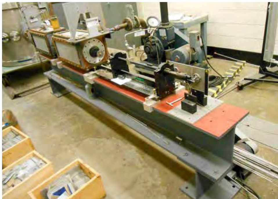
In the foreground of this photo of the Langley Miniature Light-Gas Gun, the breech of the first stage, a modified 220 Swift rifle, can be seen. In the background is an add-on vacuum chamber that was used for larger targets.
