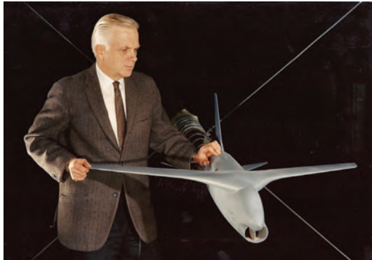
Whitcomb with modified F-8 Crusader model used to assess the performance of a supercritical wing for civil transport, 1970.
