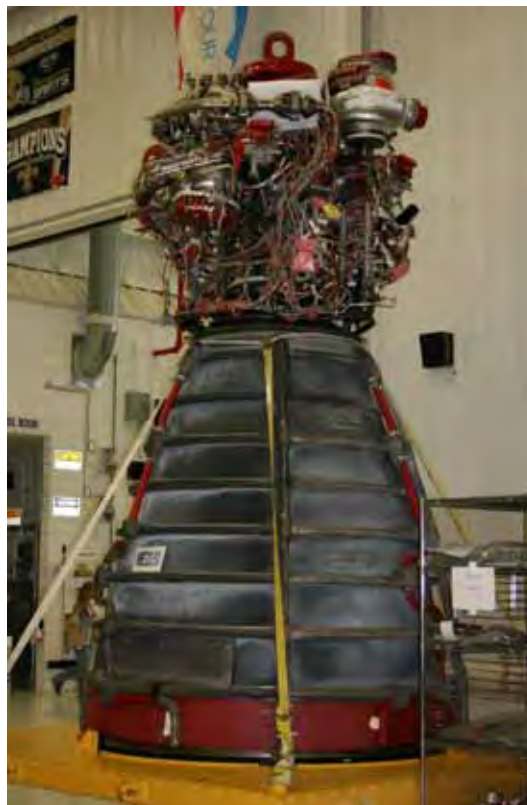
The Space Shuttle Main Engine Processing Facility refurbishes the reusable engines.
