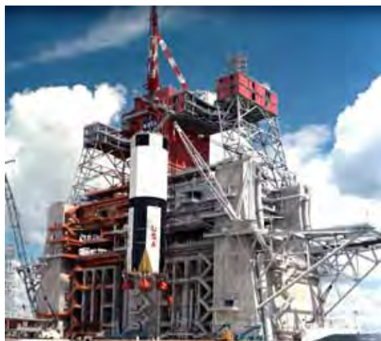
S-IC stage installation into the Hot Fire Stand at MTF, now Stennis Space Center, in 1967.
