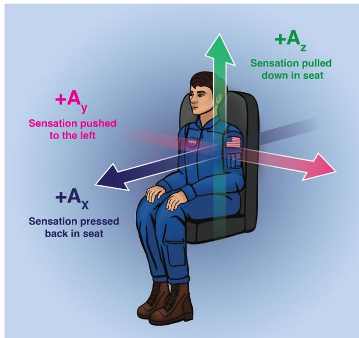
**Figure 6.5-1—Common XYZ Coordinate Frame for Translational Acceleration**
