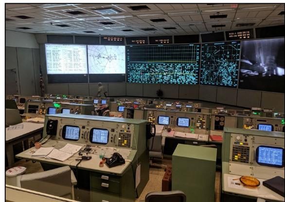
**Figure 5-10. Restored MOCR-2, showing recreated computer screens (foreground) and viewing screens (background).**
