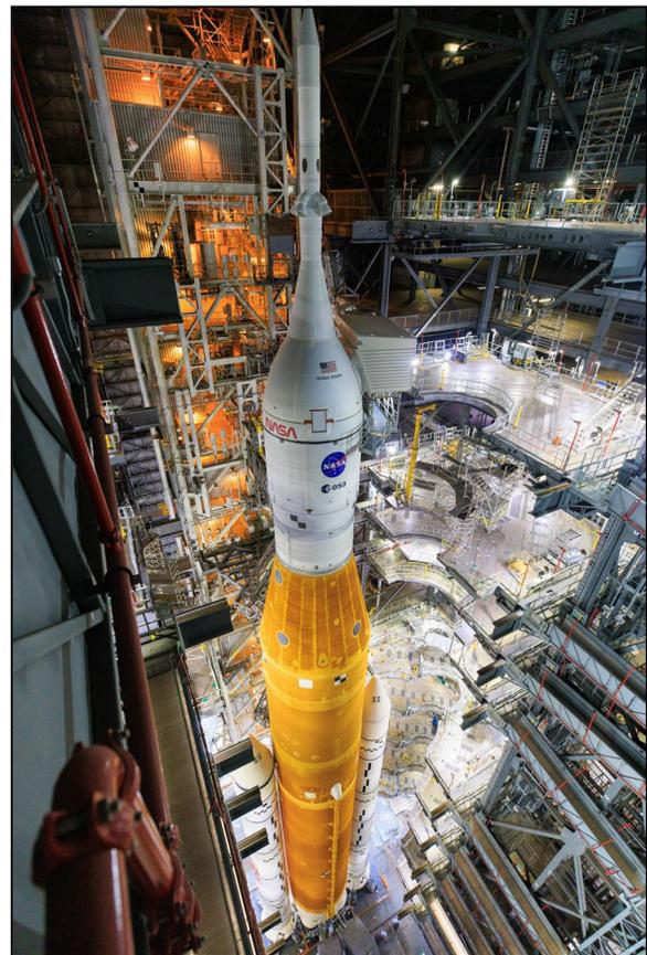
Figure 4-12. Artemis I stacked on top of the Space Launch System in High Bay 3 of the historic VAB at KSC on August 16, 2022.
