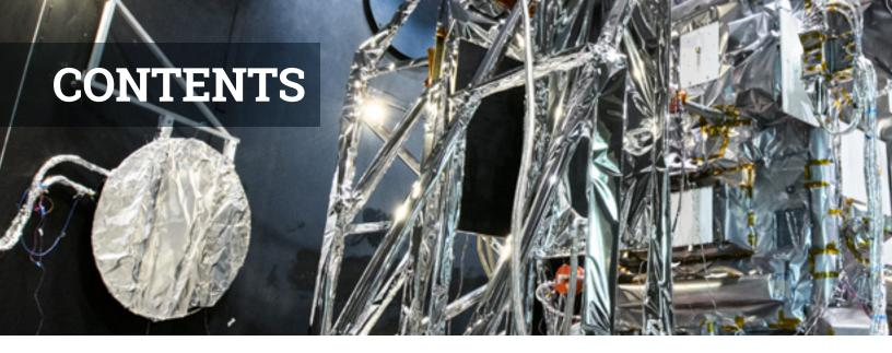
The PACE Observatory inside the SES Chamber prior to Thermal Balance Testing at NASA Goddard Space Flight Center in Greenbelt, MD. CREDIT: NASA/DENNY HENRY
