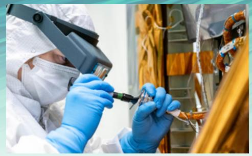
An electrical technician repairs a piece of electrical equipment on the PACE spacecraft CREDIT: NASA/KATIE MELLOS
