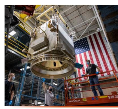
The PACE spacecraft bus with mass simulators is lifted into the Modal Facility at NASA's Goddard Space Flight Center in preparation for strength pull testing. CREDIT: NASA/DENNY HENRY
