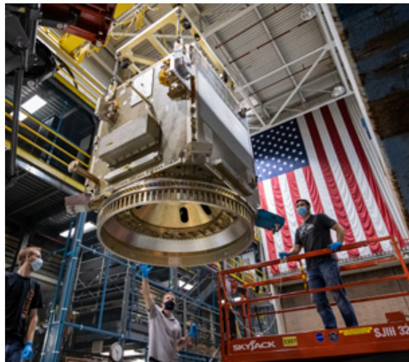
*The PACE spacecraft bus with mass simulators is lifted into the Modal Facility at NASA's Goddard Space Flight Center in preparation for strength pull testing.*
