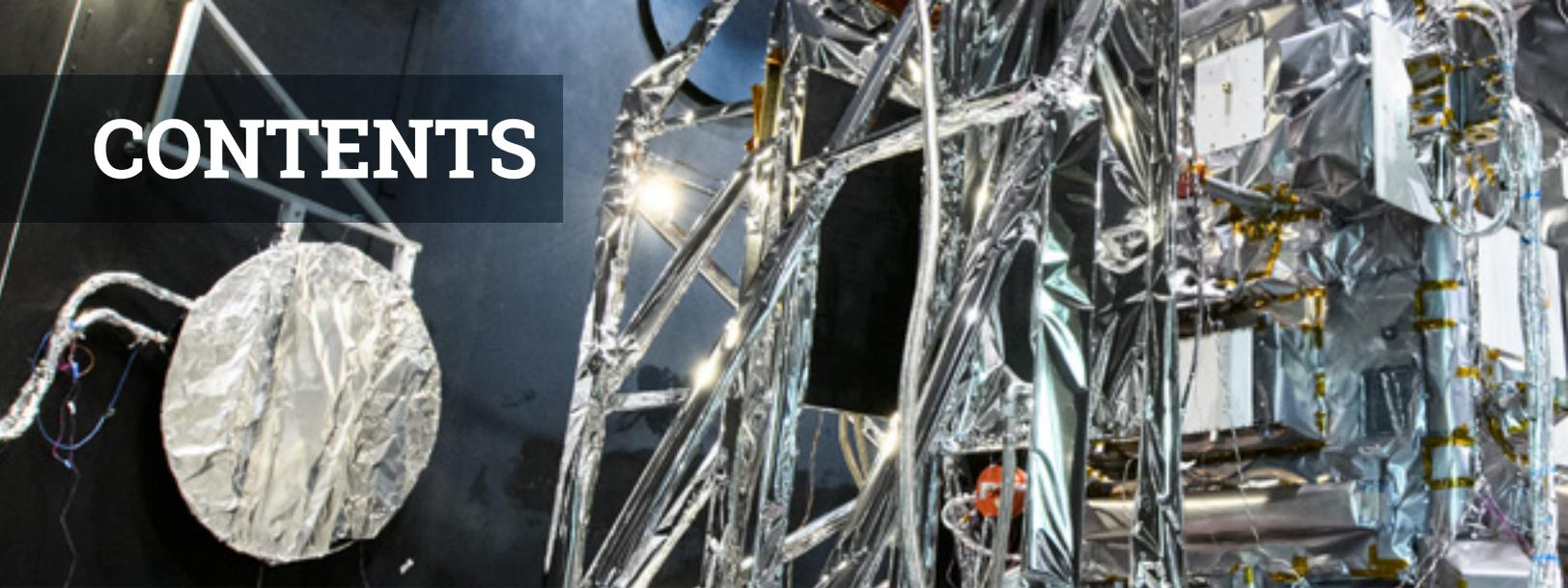
The PACE Observatory inside the SES Chamber prior to Thermal Balance Testing at NASA Goddard Space Flight Center in Greenbelt, MD. CREDIT: NASA/DENNY HENRY
