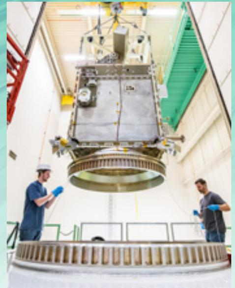
*The PACE spacecraft bus with mass simulators installed is lifted into the vibration testing facility.* CREDIT: NASA / DENNY HENRY
