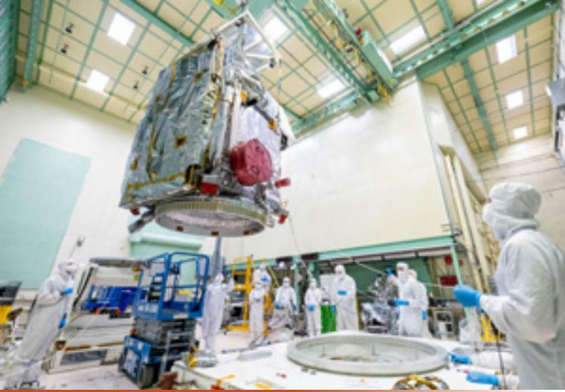
*The PACE Mechanical team performing a lift of the PACE Observatory in preparation for the Flight Solar Array Deployment. CREDIT: KATIE MELLO*
