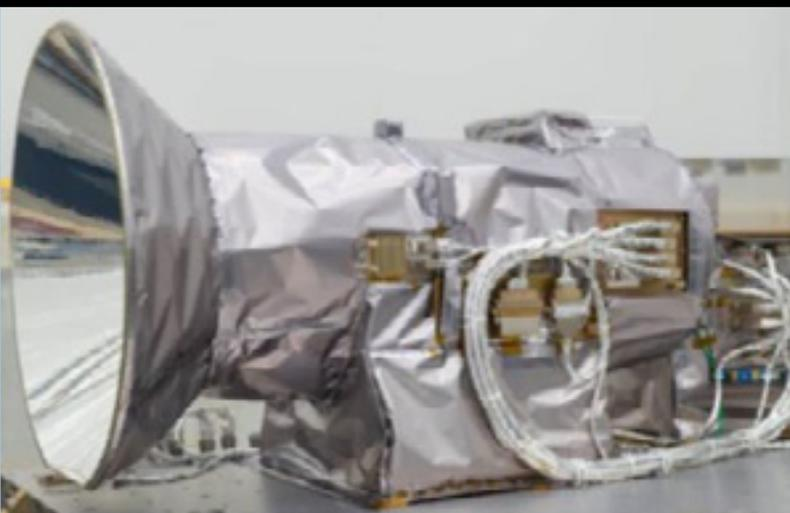
*AWE Instrument, the Advanced Mesospheric Temperature Mapper (AMTM)* CREDIT: NASA/SDL
