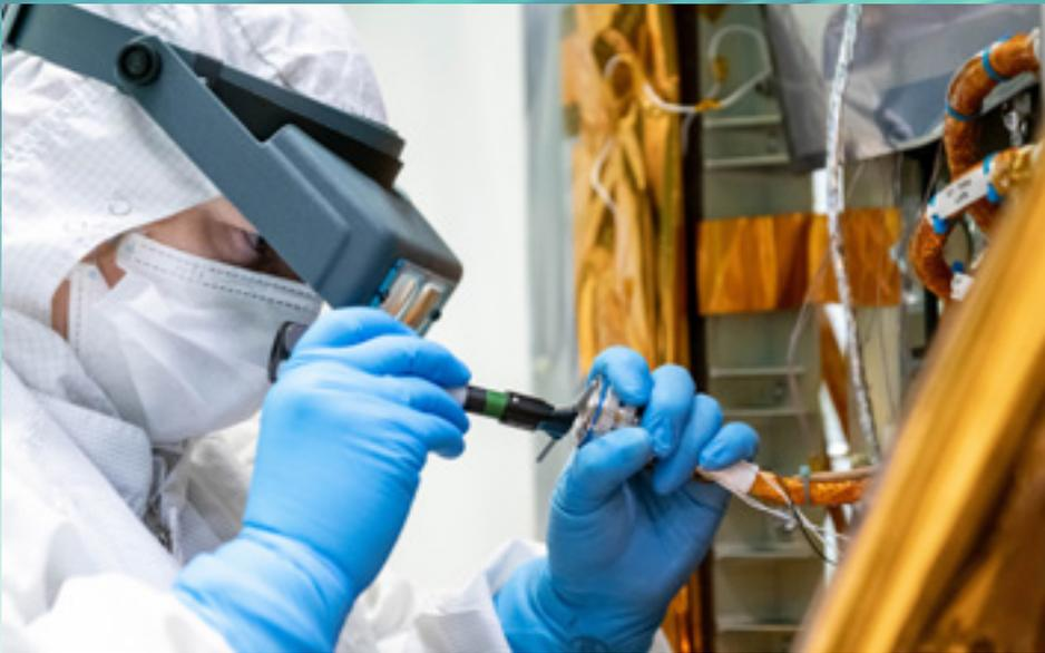
*An electrical technician repairs a piece of electrical equipment on the PACE spacecraft* CREDIT: NASA/KATIE MELLOS
