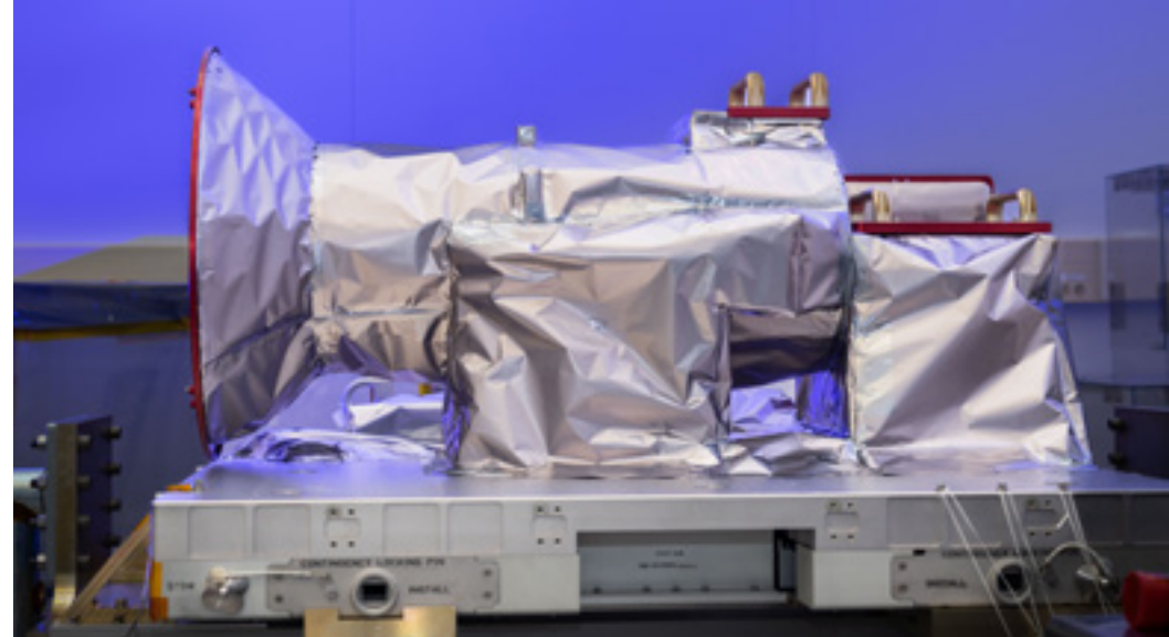
AWE instrument installed on the ExPA. Red fixtures protect crucial areas and will be removed prior to launch. CREDIT: SDL
