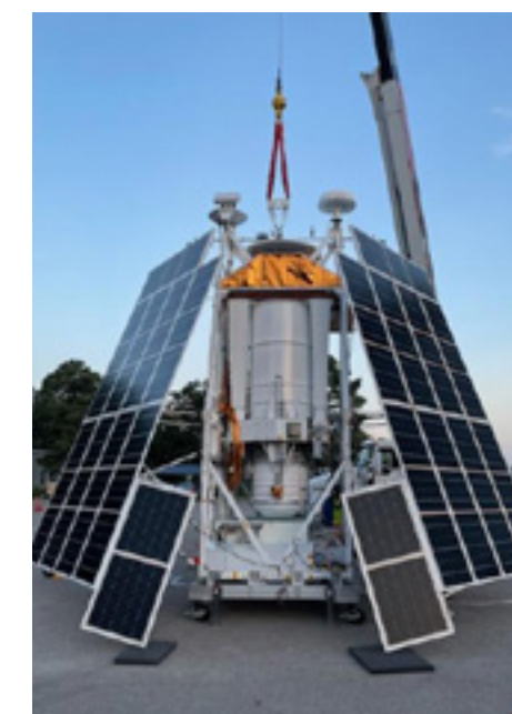
GUSTO Observatory During Compatibility (Hang) Test, August 10, 2023, at CSBF. CREDIT: NASA/MICHAEL SILBER
