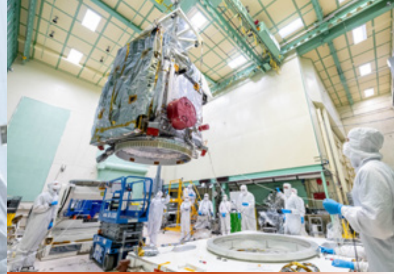
The PACE Mechanical team performing a lift of the PACE Observatory in preparation for the Flight Solar Array Deployment. CREDIT: KATIE MELLOS
