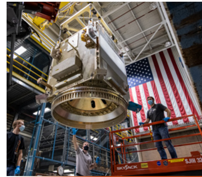
The PACE spacecraft bus with mass simulators is lifted into the Modal Facility at NASA's Goddard Space Flight Center in preparation for strength pull testing. CREDIT: NASA/DENNY HENRY
