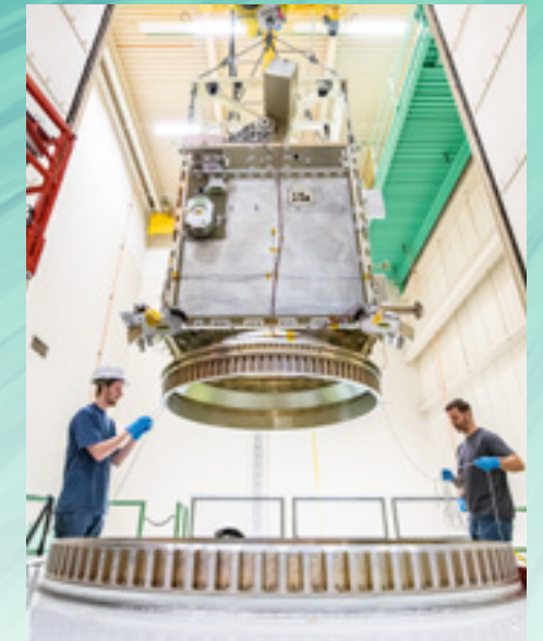
The PACE spacecraft bus with mass simulators installed is lifted into the vibration testing facility. CREDIT: NASA / DENNY HENRY
