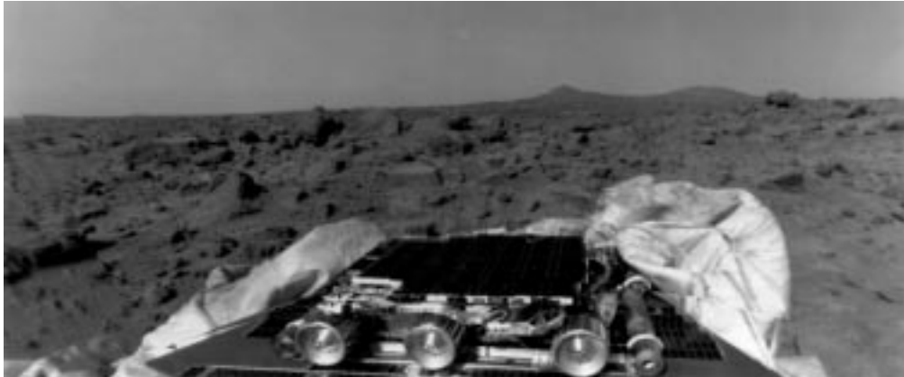
The Sojourner rover and undeployed ramps onboard the Mars Pathfinder spacecraft can be seen in this image taken by the Imager for Mars Pathfinder on July 4, 1997.
