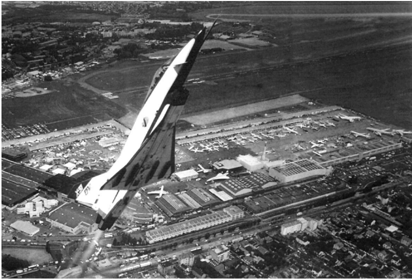
The joint X-31 enhanced fighter maneuverability program involved the Navy, Air Force, NASA, Rockwell International, the German Defense Ministry, and Daimler Benz Aerospace. This two-aircraft program set a new X-plane productivity record and assessed the impact of thrust vectoring during slow-speed, poststall maneuvering.
