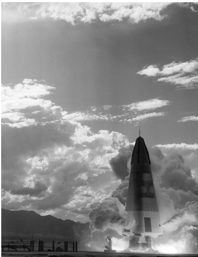
The Air Force's Phillips Laboratory conducted test flights using the McDonnell Douglas Delta Clipper–Experimental (DC-X) launch vehicle. The DC-X was designed as a simplified demonstration vehicle to test concepts that would be necessary for a cost-effective reusable launch vehicle. In FY 1995, the Air Force transferred the DC-X to NASA to be upgraded for additional flight tests in 1996 as the DC-XA (Delta Clipper–Experimental Advanced).
