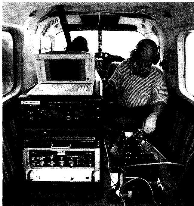
Airborne Laser Profilers used by the Forest Service and Agricultural Research Service to study changes in landscape patterns due to erosion and other activities of man.
