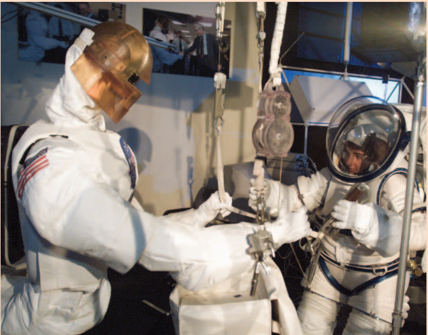
Astronaut Nancy Currie participates in a test with Robonaut, NASA's dexterous robotic assistant, to evaluate human-robotic operations. NASA is developing a wide range of autonomous robotics that will conduct surveys in advance of human exploration, offer astronauts an extra set of "hands and eyes," and conduct operations that would be hazardous to humans.
