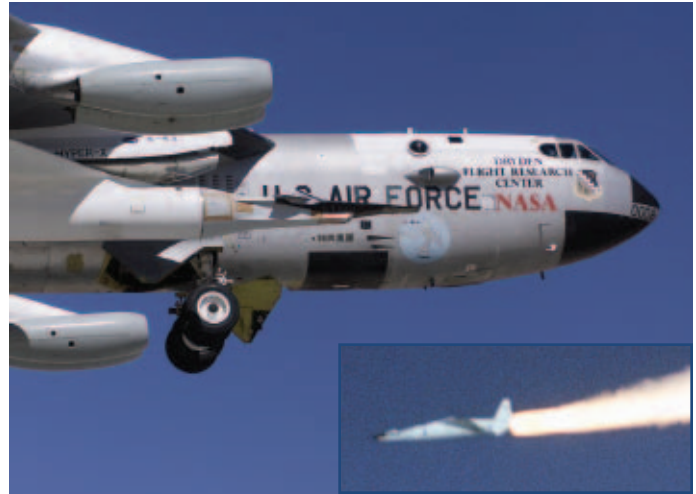
Tucked under the wing of NASA's B-52B aircraft, the X-43 hypersonic research vehicle performed a captive carry evaluation flight on September 27, 2004. It is powered by a revolutionary supersonic-combustion ramjet, or "scramjet." Inset: The X-43's rocket ignited moments after release from the B-52B, setting the vehicle on a record-setting flight where it reached nearly Mach 9.8 (7,000 miles an hour). NASA is developing scramjet technology to carry vehicles from Earth to orbit without the heavy oxygen tanks carried by currently-used launch vehicles. Credit: large photo, T. Tschida.
