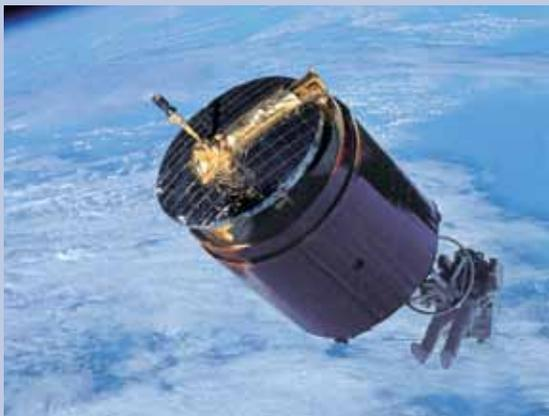
Figure 1.6 – Palapa B2 Recovery – Palapa B2 being manipulated by an astronaut in a free-flying Manned Maneuvering Unit. Palapa B2 was returned to Earth for refurbishment and eventual reflight.
