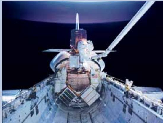
Figure 1.5 – Solar Maximum Mission in the Space Shuttle Bay – The Solar Maximum Mission was one of the first orbiting spacecraft to be retrieved, repaired, and redeployed using satellite servicing. This photograph from 1984 shows the spacecraft being repaired by astronauts in the payload bay of the space shuttle Challenger.
