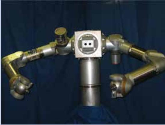
Figure 4.6 – Ranger Telerobotic Shuttle Experiment – The Ranger dexterous manipulator pair mounted to a head that is attached to a positioning leg. This hardware was designed to be positioned at a worksite using a grapple arm or a positioning leg.
